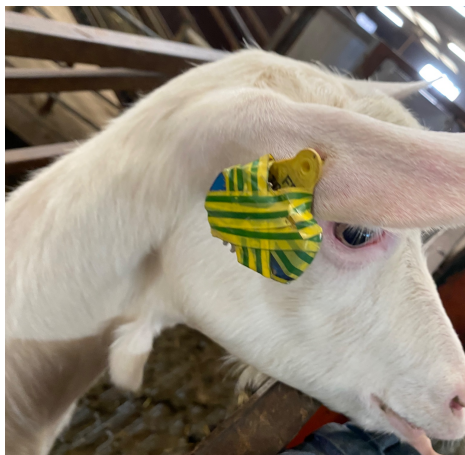
Figure 1 - A goat with an accelerometer fixed with tape to the right RFID ear tag in lateral view.
